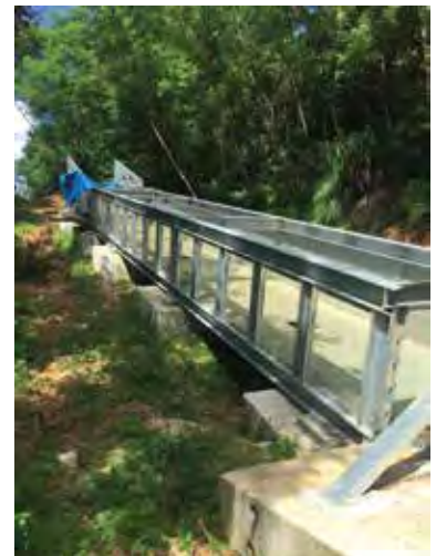
A 20-m-long flume model to study the fundamental interaction mechanisms between landslides and barriers at the Kadoorie Centre.
